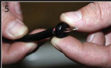
5 Place the tulle over the cable
