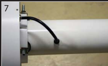
7 Press the tulle tightly in the pole
