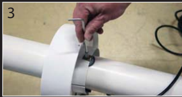
3 Clamp the unit with the bolts with hexagon tool nr. 4. When inner diameter is too small, use included bolts from the outside to clamp the fixture
